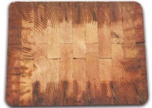
Typical treatment penetration at groundline.
