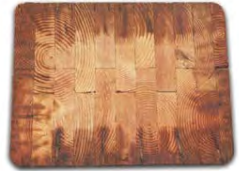
Typical treatment penetration at groundline.
