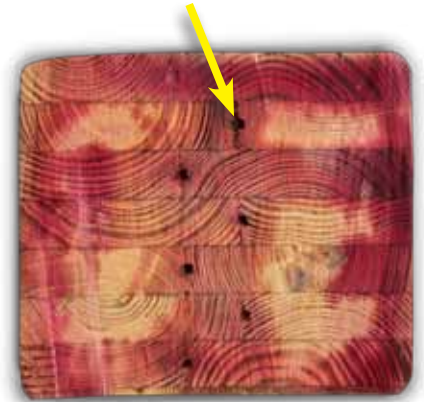
Typical treatment penetration throughout entire length of the pole.
