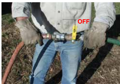
Connect air supply hose to the inline safety valve. Valve should be in the OFF position (See caution note).
