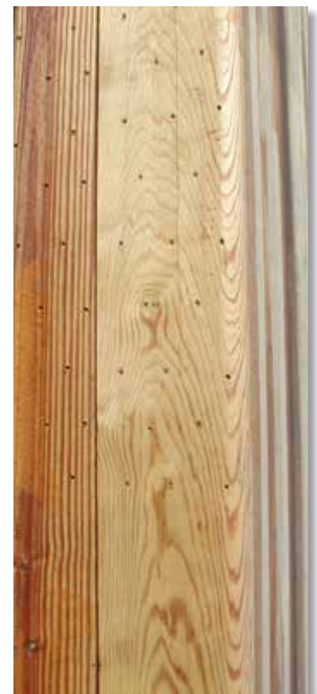
Groundline deep boring.
