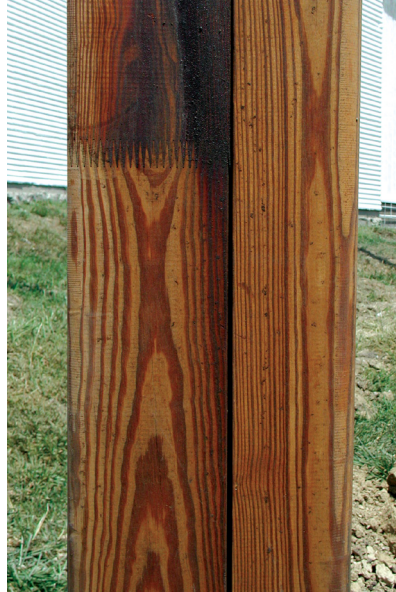
Photo B – Typical unglued edge joint on uncut side of pole which runs the entire length of pole.
