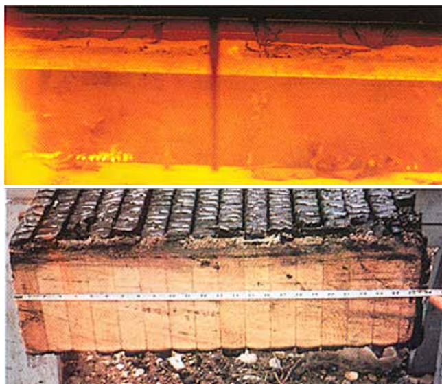
Glulam laminated wood sample during (top photo) & after (above photo) ASTM E-119 fire exposure test.
